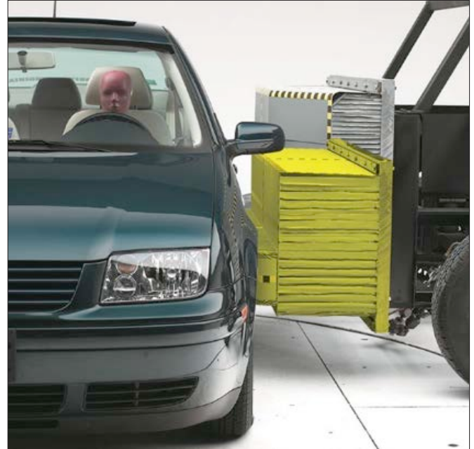
A side crash test comparison – the NHTSA barrier is shown in yellow while the taller IIHS barrier at the rear is gray. (Image: IIHS)
