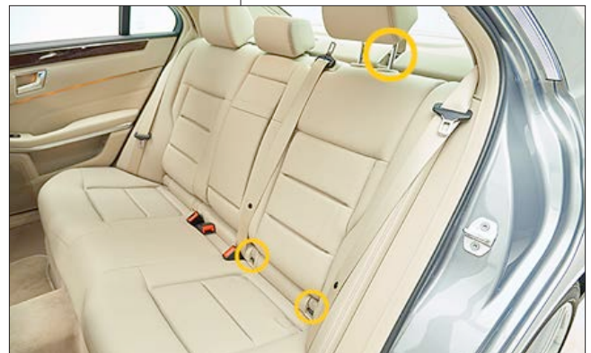
Anchor and tether locations on a typical vehicle rear seat. (Image: IIHS)
