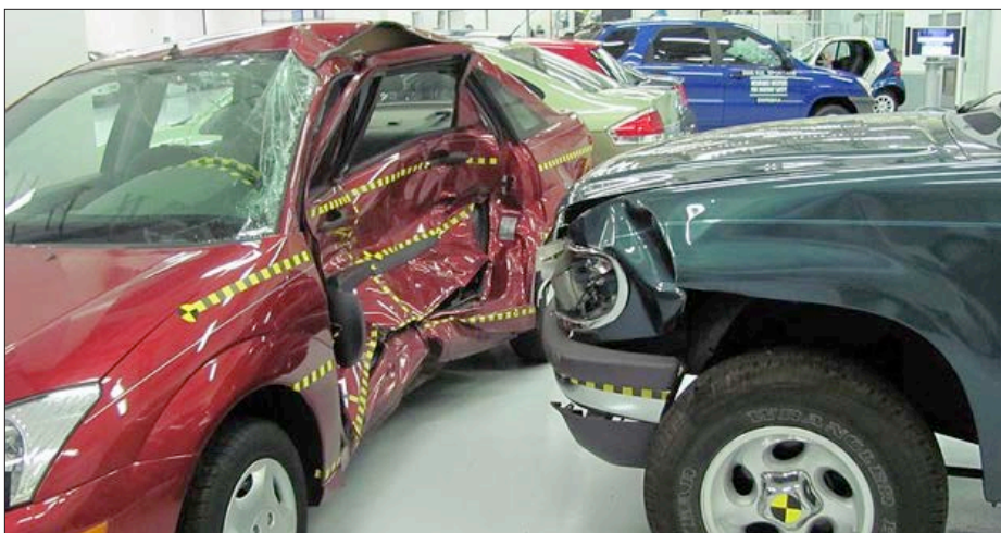
The outcome of a side impact crash test. (Image: Brady Holt, CC BY 3.0)
