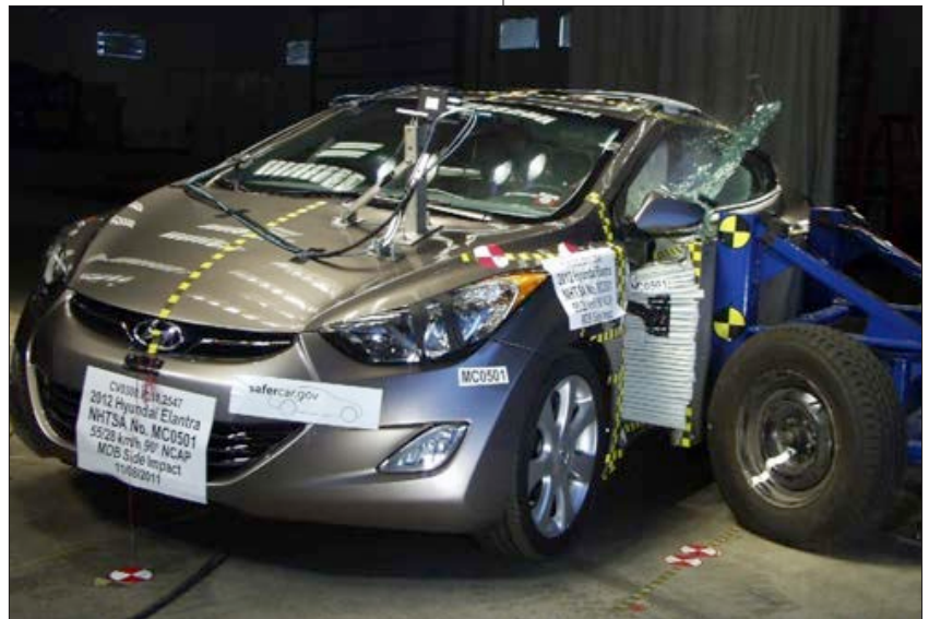
A Hyundai Elantra side barrier crash test. (Image: NHTSA)
