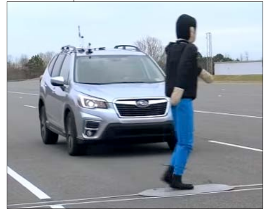
A dummy being pulled in front of a moving vehicle for IIHS pedestrian detection testing. (Image: IIHS)
