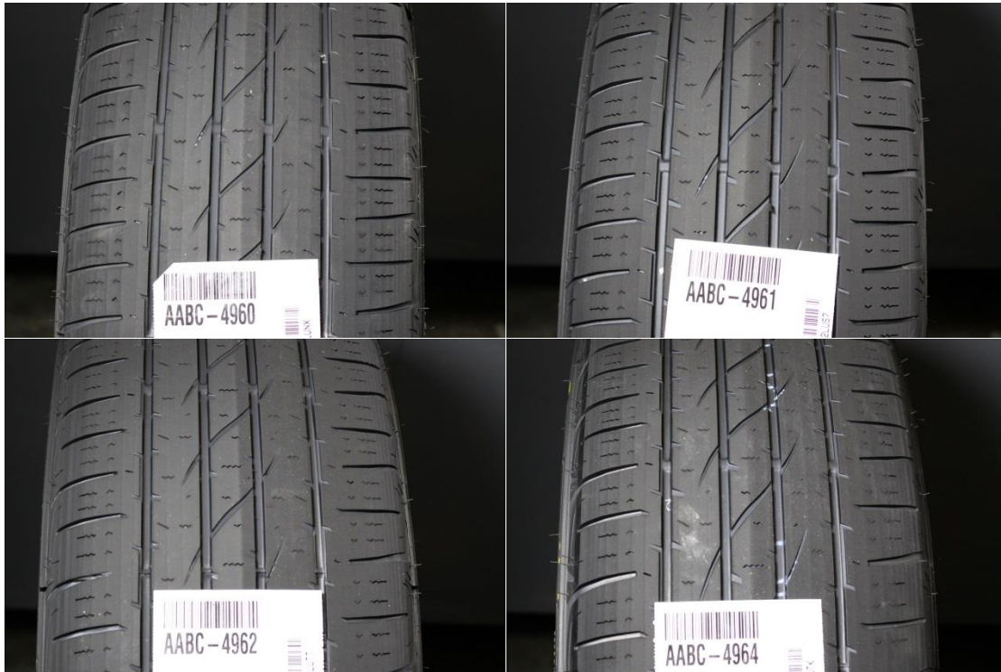
Figure 79. Buffed Tire Photos: Firestone Destination LE2 (LI=113T) Image Source: AAA
