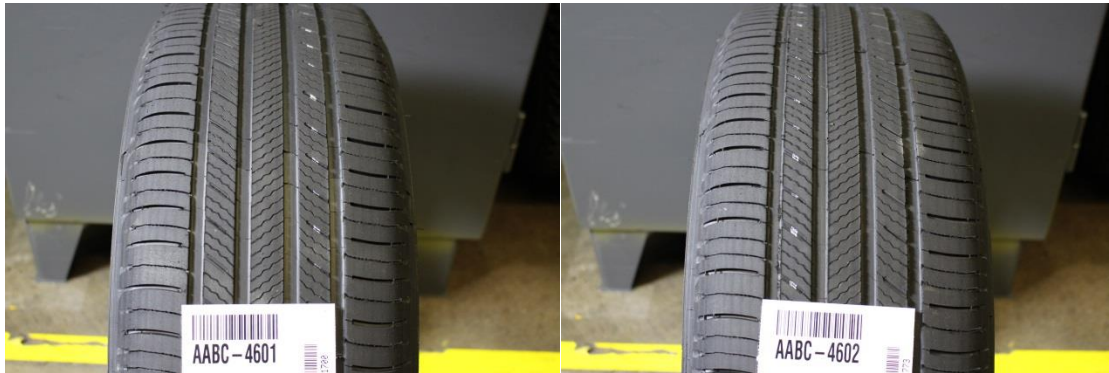
Figure 65. Buffed Tire Photos: Michelin Premier A/S Image Source: AAA
