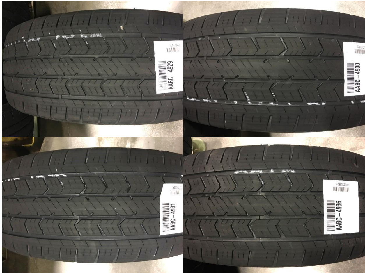
Figure 73. Buffed Tire Photos: Cooper Evolution H/T (LI=115T) Image Source: AAA
