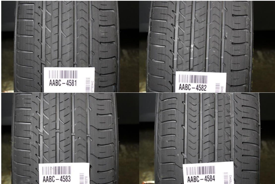
Figure 63. Buffed Tire Photos: Goodyear Eagle Sport A/S Image Source: AAA
