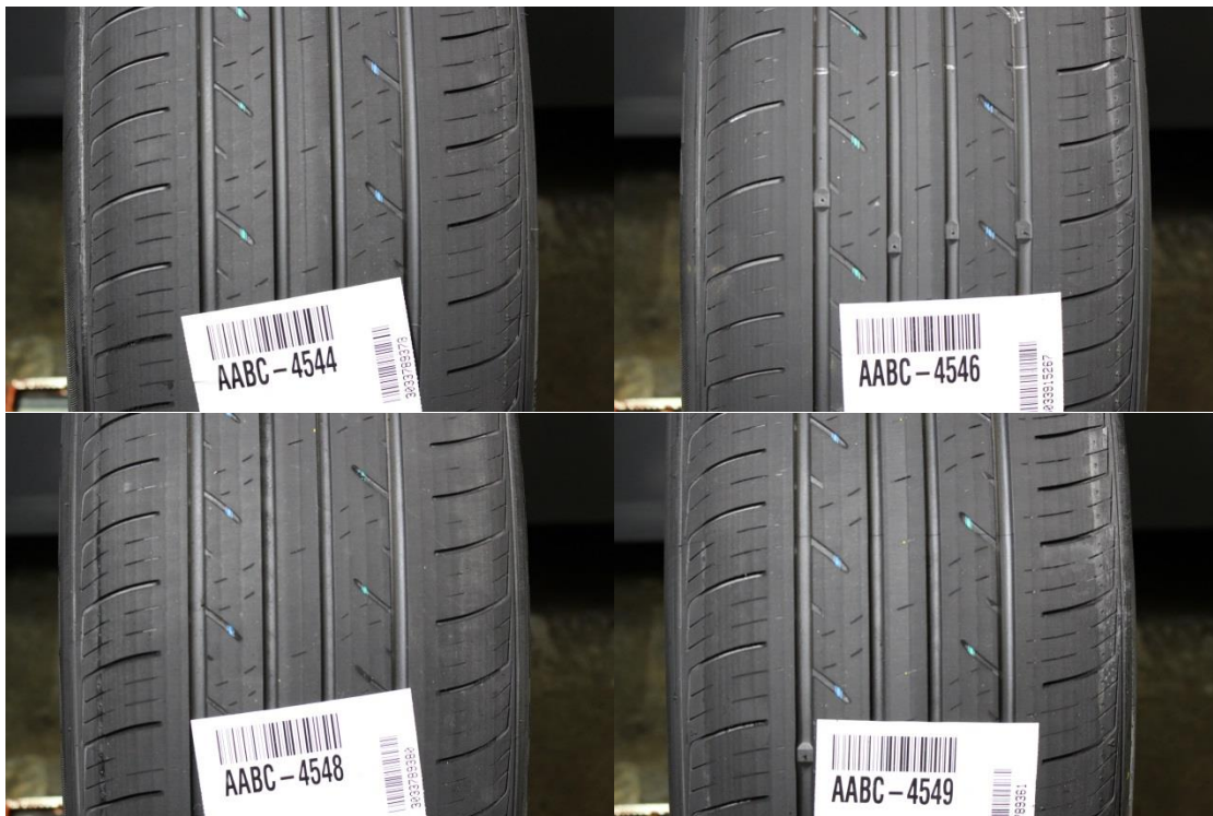
Figure 59. Buffed Tire Photos: Nexen Classe Premiere CP671 Image Source: AAA
