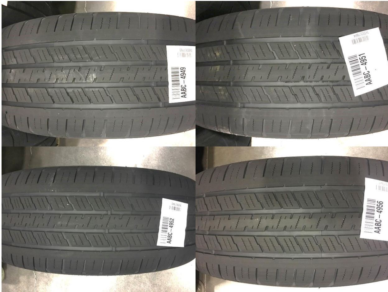
Figure 77. Buffed Tire Photos: Hankook Dynapro HT RH12 (LI=113T) Image Source: AAA
