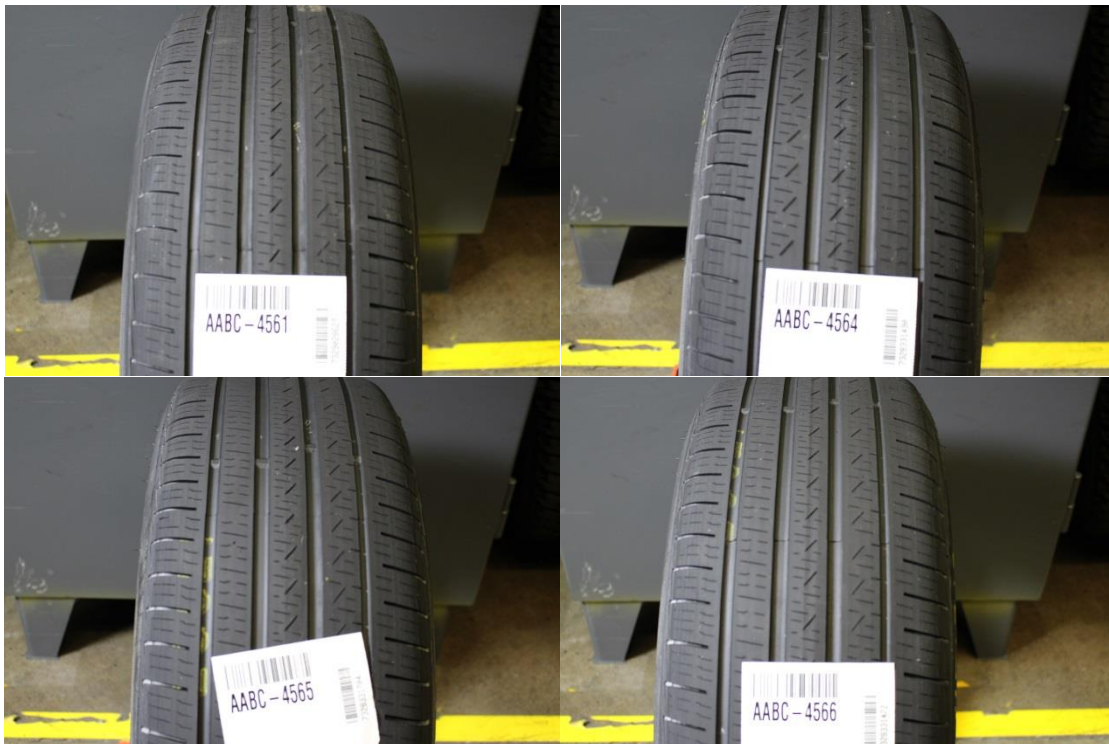
Figure 61. Buffed Tire Photos: Pirelli Cinturato P7 A/S+ Image Source: AAA
