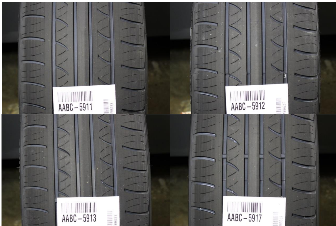
Figure 69. Buffed Tire Photos: Fuzion Touring Image Source: AAA
