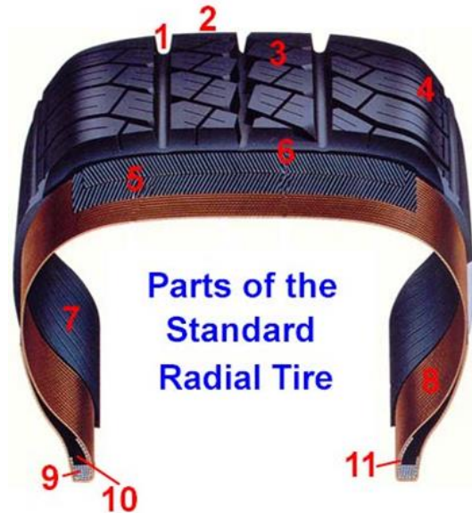
Figure 2: A cutaway view of a typical radial tire Image Source: Tire Guides Inc.
