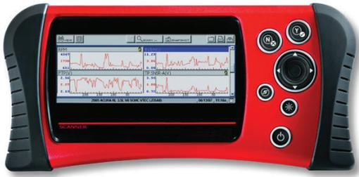
To access DTCs, technicians connect a “scan” tool to a Diagnostic Link Connector that is commonly located under the driver’s side of the instrument panel. The scan tool displays any stored codes, and many motorists think that’s where diagnosis ends. They question why they should have to pay, sometimes dearly, for such a simple procedure.
