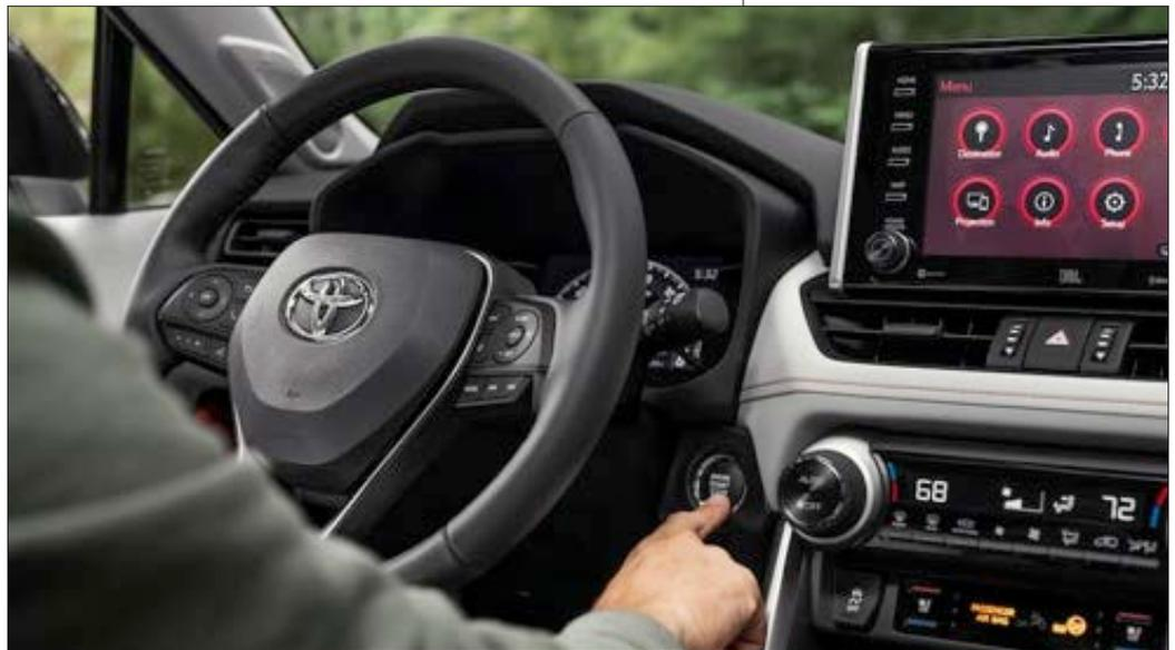
**A maintenance reminder reset on this Toyota requires pressing the ignition and trip meter buttons in a specific sequence. (Image: Toyota)**
