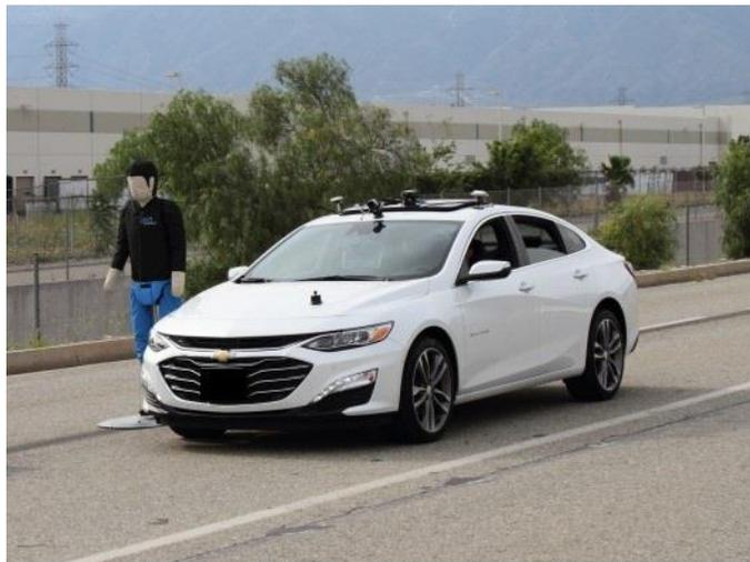
**Figure 3: 2019 Chevrolet Malibu outfitted with measurement equipment** Image Source: AAA
