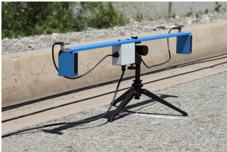
**Figure 7: 4active light barrier for pedestrian target timing** Image Source: AAA
